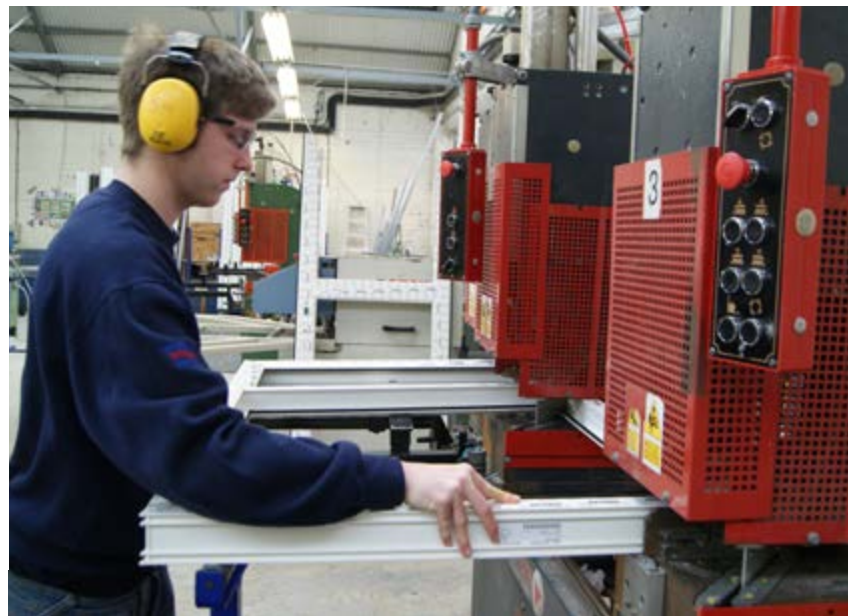
Joe Hunter welding frames in our state-of-the-art factory
